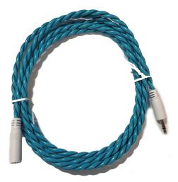
The perimeter cable allows an ultra-precise detection of the least drop of water thanks to an advanced technology and a helicoidal structure composed of anticorrosive materials. As soon as any conductive liquid has been detected (water, weak acid and base) a signal is transmitted to a wireless probe that will carry the signal to the control unit.
